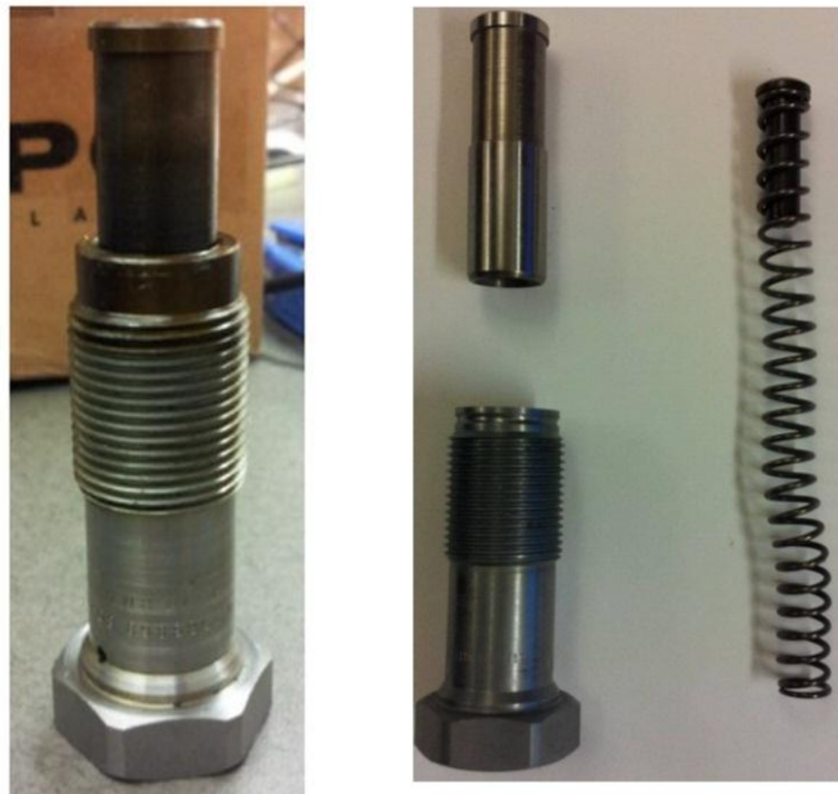
Figure 2: Timing Chain Tensioner Assembled (left) and Disassembled (right)
