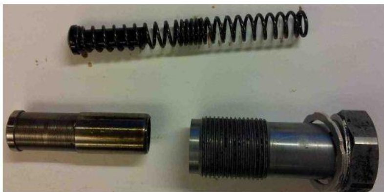
Figure 5: Disassembled Used Timing Chain Tensioner
