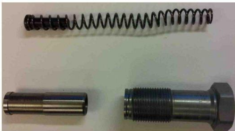
Figure 6: Disassembled New and Unused Timing Chain Tensioner
